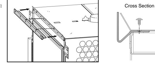
To attach the Inset Fascia a magnet bracket must be fixed to the firebox. This bracket slides in to sit flush with the underside of the top firebox panel. To secure it in place screw the provided pozi-drive screws into the four holes, positioned behind the 45 degree flange at the top edge of the firebox.
